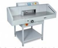
The Formax Cut-True 29A Electric Guillotine Paper Cutter offers precision cutting for paper stacks up to 20.5" wide. User-friendly, intuitive features include a touchscreen control panel, automatically-adjusting back gauge and the capacity to program up to 100 jobs/100 cuts. An infrared light beam safety curtain provides safety and convenience as it shuts down operation if the light plane...
