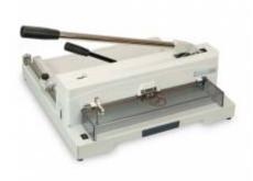
The Cut-True 13M Tabletop Manual Paper Cutter is rugged and compact with a hardened steel blade and LED Laser Line for precision cutting with minimal effort. Simply load a stack of paper, up to 14.5" wide, secure with the clamp, and pull down on the lever arm; it's that easy. The back gauge and calibrated scales allow operators to make fine adjustments, while the Laser Line shows...
