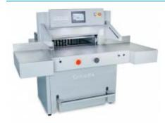
The Cut-True 31A Electric Guillotine Paper Cutter offers precision cutting for paper stacks up to 28" wide, up to 4" high. User-friendly, intuitive features include a 7" color touchscreen control panel, automatically-adjusting back gauge and the capacity to program up to 100 jobs/100 cuts. An infrared light beam safety curtain provides safety and convenience as it shuts down...
