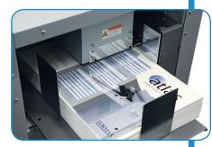
Upper-belt tri-suction feed system for accurate feeding of large & heavy stocks
