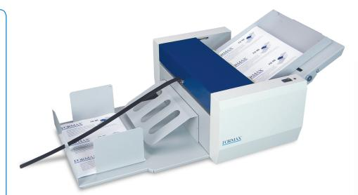
The **FD 90 Rotary Perforator/Creaser** is specially designed for finishing printed sheets, up to 13.8" x 19". Its three-tire friction feeding system reliably feeds up to 6,800 sheets per hour, and can create up to 5 parallel perforations and/or creases in a single pass. Perforating allows for easy separation of multiple printouts, tear-offs, postcards or tickets on a single sheet, while creasing allows for easy folding and reduces unsightly cracking in digital printouts.
